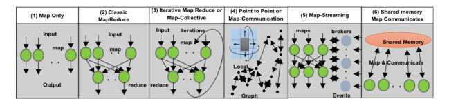
Figure 2: Six Distinctive Software/Hardware Architectures for Data Analytics
